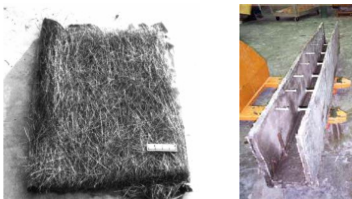
Fig. 1 SIMCON: Continuous fibre-mat; SIMCON stay-in-place formwork.
