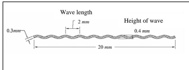
**Fig. 1** Optimized crimped fibre
