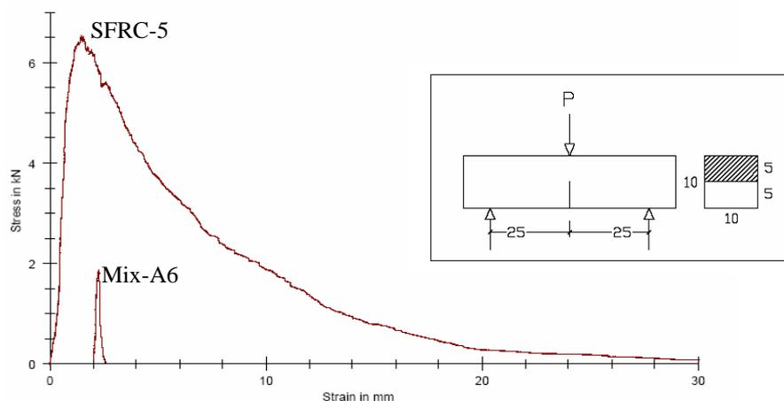
**Fig.2** Comparison of behaviour of FRC and matrix notched beam under three-point bending
