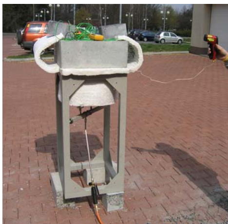
Figure 1 Location of the concrete panel in a heating bench pickups
