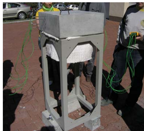
Figure 2 Temperature sensing in elements by means of sensors and pickups
