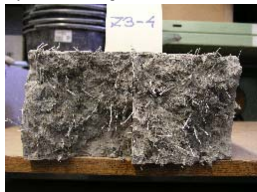
Fig. 2 Pulled fibres on the sample surface
