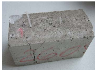
Fig. 5 BeneSteel W pull-out test
