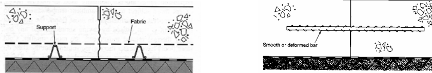
Fig. 7 Sawn and formed restrained joint
