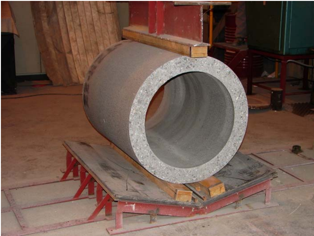
Fig. 5 Testing of the sewer pipe
