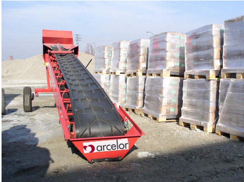
Fig. 3 Conveyor belt for dosing fibres
