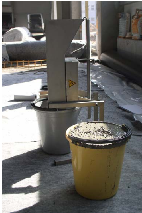
Fig. 1 The Dosometer and sample of concrete mixture before test
