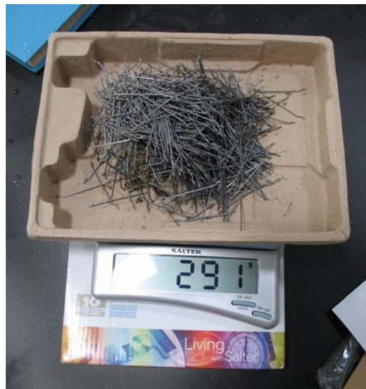
Fig. 2 Cleaned and dried steel fibres, separated from SFRC mixture using the Dosometer device
