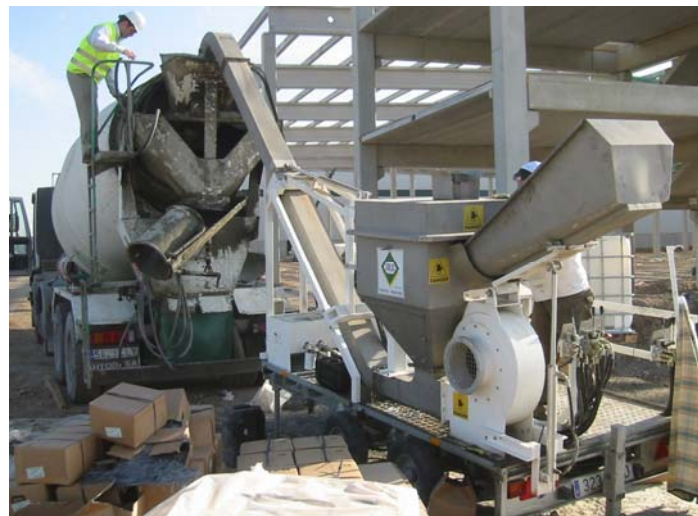
Fig. 4 Blast machine for dosing fibres by airflow
