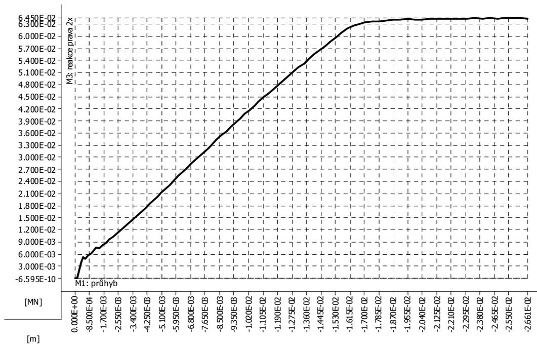
**Fig. 7 Diagram of total load vs. deflection in the simulated four-point bending test**
