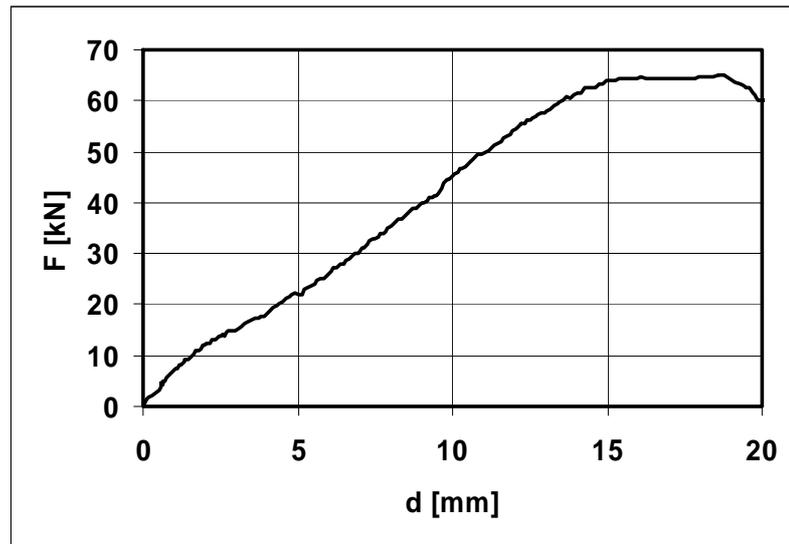
**Fig. 3 Measured load-deflections response of the beam**
