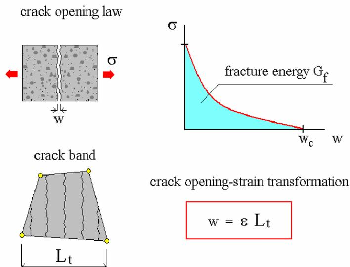
**Fig. 5 Smeared crack model for tensile behavior of concrete**
