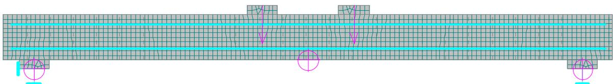
**Fig. 6 Finite element model of the four-point bending beam with reinforcement, boundary conditions and measurement points**
