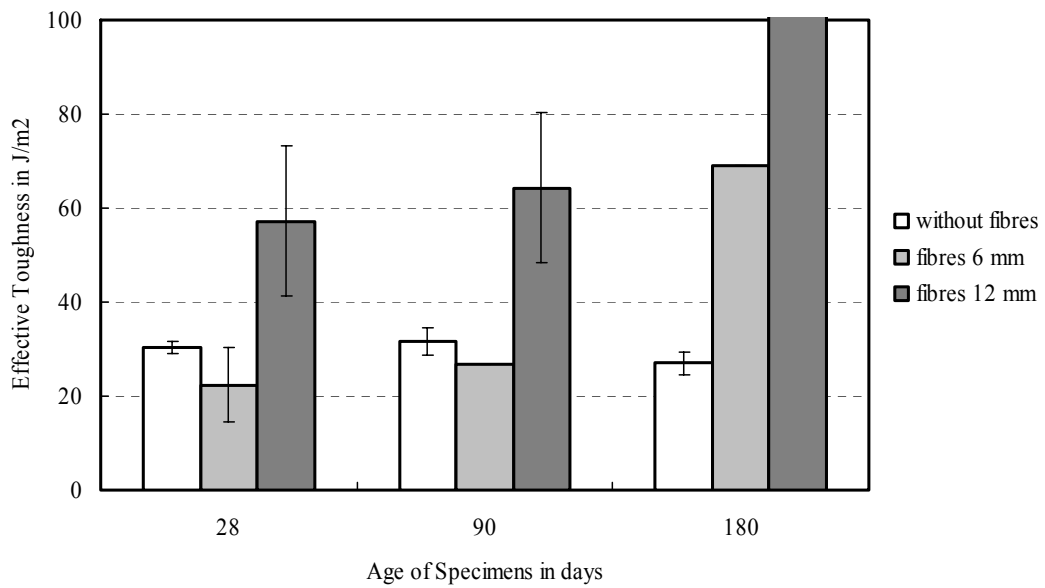
Fig. 2b Effective toughness vs. age of specimens (detail)
