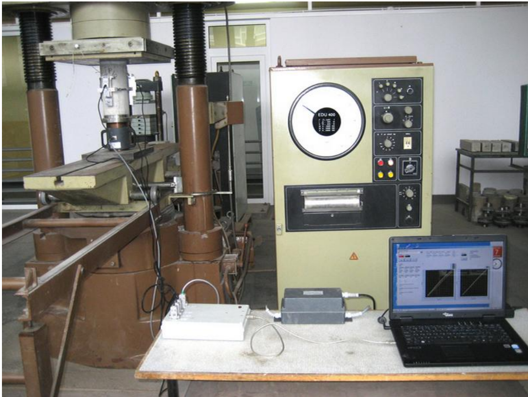
Fig. 1 Measurement equipment for \sigma - \varepsilon relationship and modulus of elasticity.
