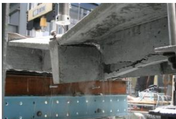
Fig. 3 Destruction of the specimen.
