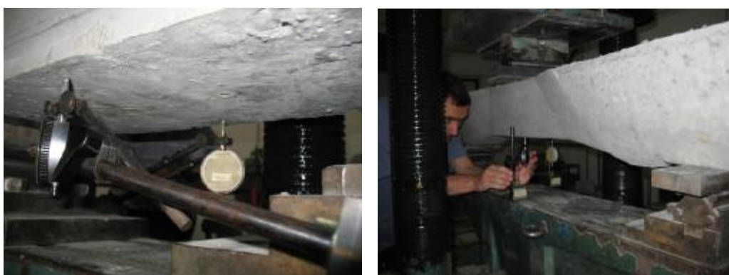
Fig. 2 Detail of the test configuration of the sleeper – three-point bending of the cross-section under the rail (left) / in the middle; indicator clocks for deflection measurement are installed on both sides of the sleeper
