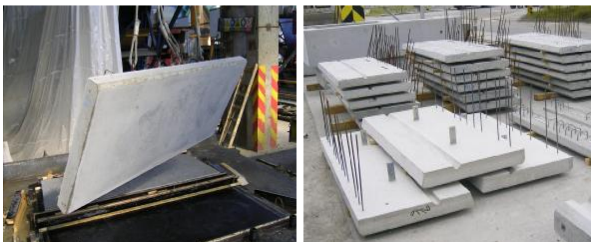
Fig. 4 and Fig . 5 Front side of the hardened cornice plate and a factory stock-yard
