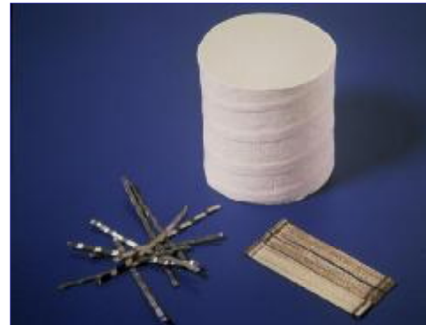
Fig. 5 Fibers loose, circumferentially wrapped, and glued side by side
