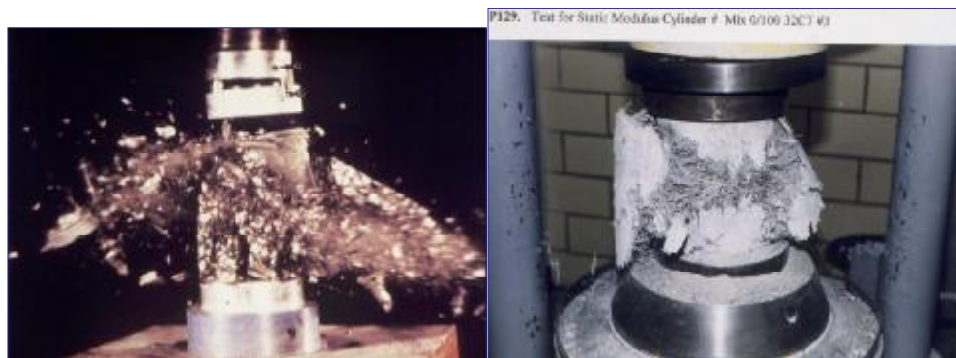
Fig. 2 No fiber concrete cylinder break Fig. 3 – FRC extended cylinder break
