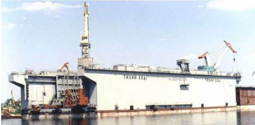
Fig. 4. The floating dock with load-carrying ability of 8,000 tons.
