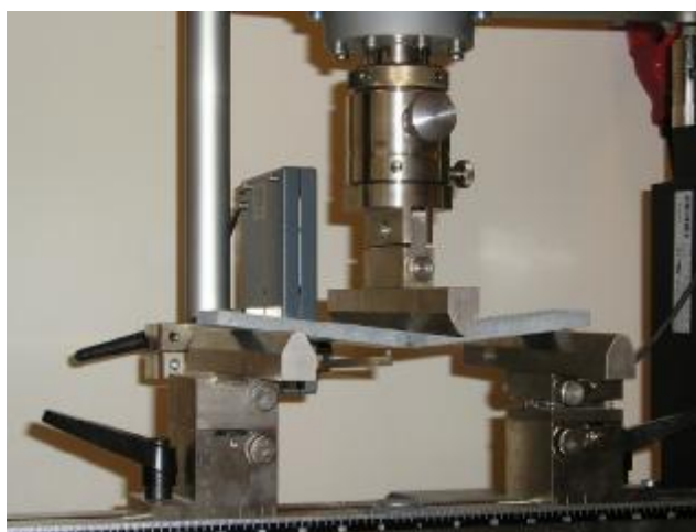
Fig. 1 Configuration of the three-point bending test
