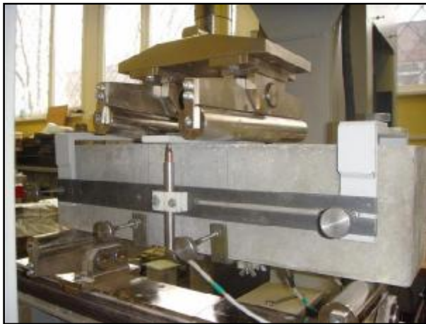
Fig. 1 Fiber concrete prism 4-point bending test.
