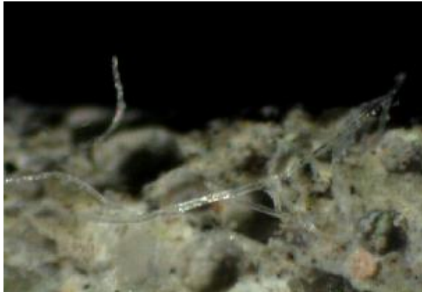
Fig. 3 Close up of PP fiber in cement matrix without deterioration – sample not exposed to heat
