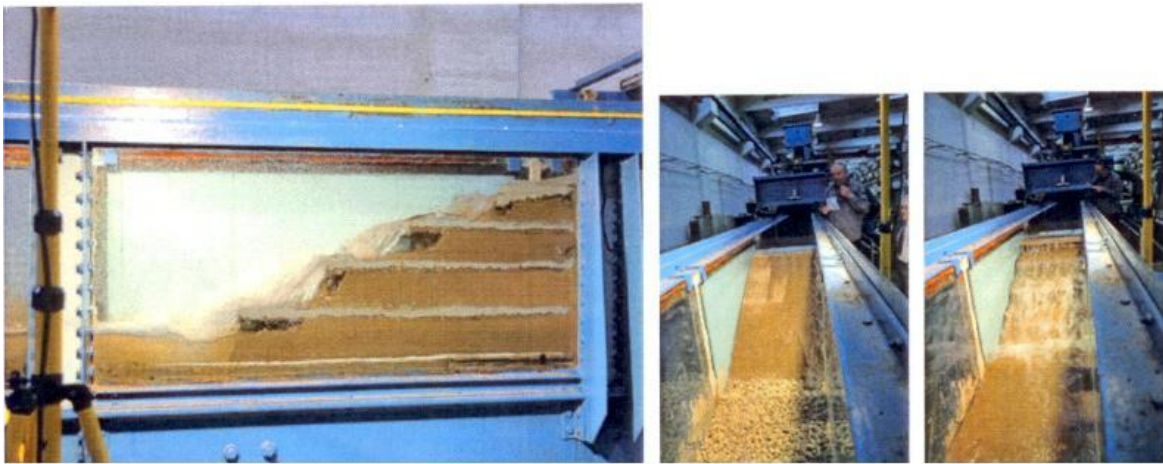
Fig. 7 Laboratory model of dam with inserted fibre concrete slabs.
