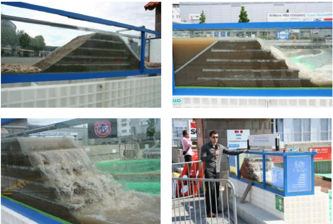
Fig. 7 Laboratory model of dam with inserted fibre concrete slabs.
