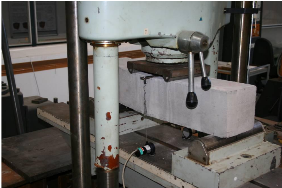
Fig.3: Scantling after the test (at ambient temperature)
