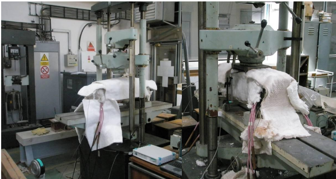
Fig. 7: The specimen during the heating
