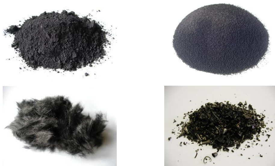
Fig. 1: Electrically conductive materials: micronized graphite, expanded graphite, carbon fibres, metal parings
