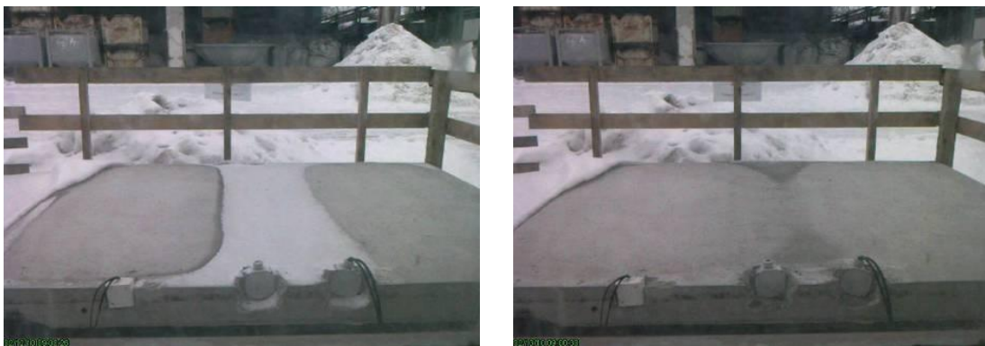
Fig. 10: Operation of the tempered panel in real conditions
