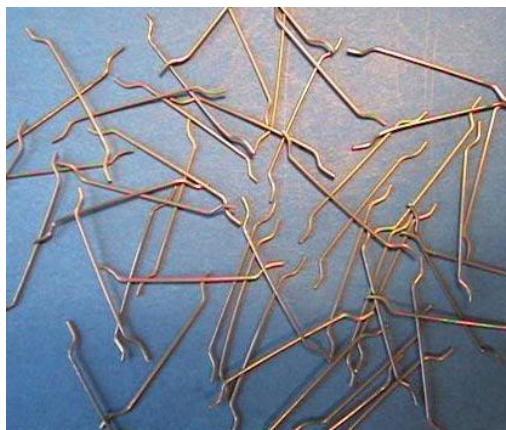
Fig 3. Steel fibres (SI Concrete systems 2003)
