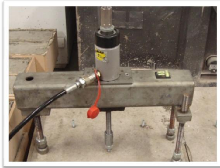
Fig. 7: Anchor pullout apparatus
