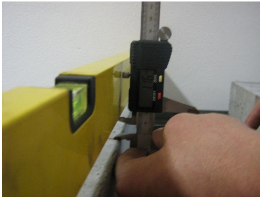
Fig. 8: Measuring of the increase of deformation
