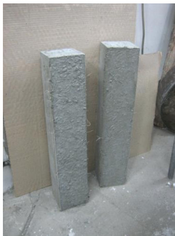
Fig. 2: Picture of the manufactured specimens 150x150x700 mm
