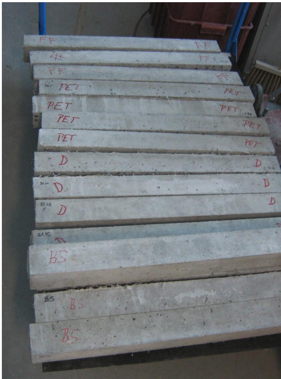
Fig. 3: Picture of the specimens for experiments 75x75x700
