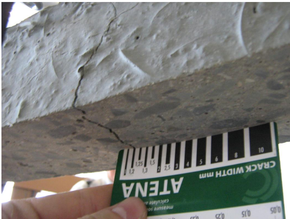
Fig. 5: Control measuring of the crack width after three-point bending test
