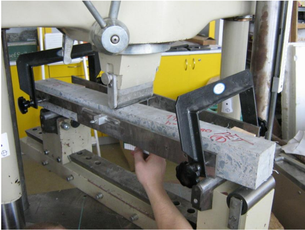
Fig. 4: Creating of a flexural macro-crack in a three-point bending test
