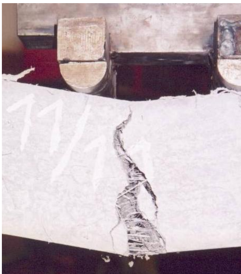
Fig. 1: Bridging of fibres across the macro-crack
