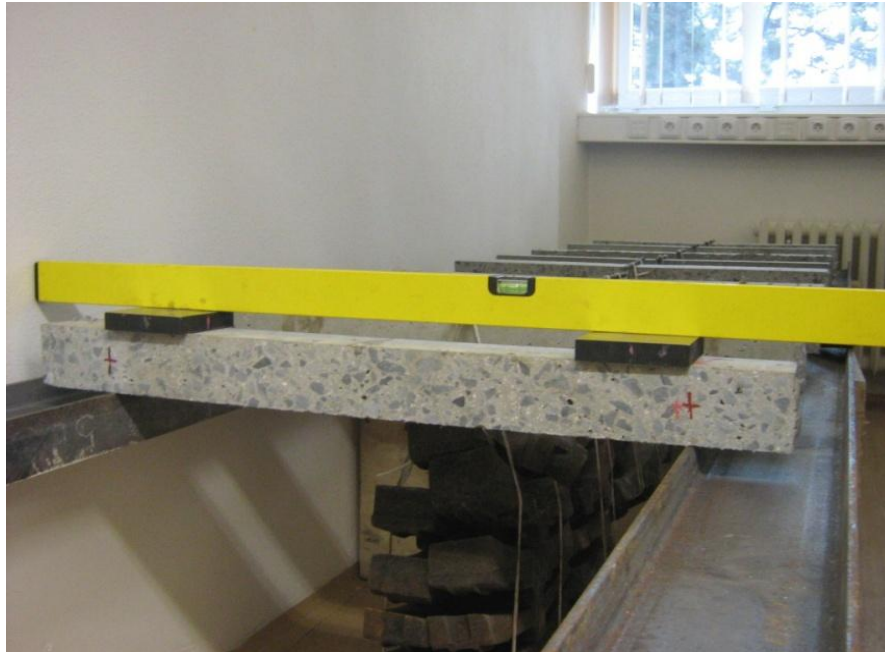
Fig. 7: Measuring of the initial deformation before the long-term loading of the specimen
