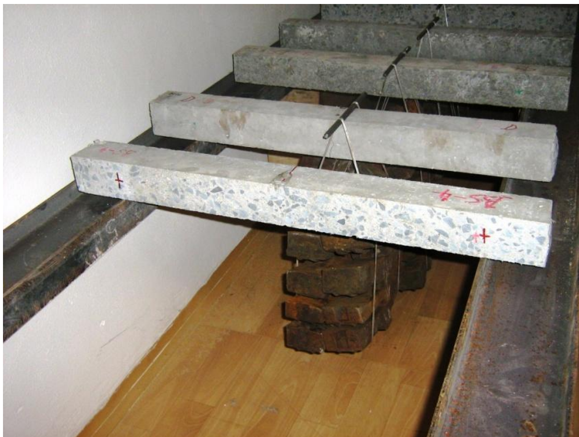
Fig. 6: Specimens with long-term load
