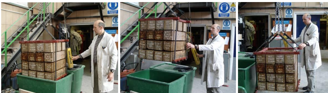
Fig. 4: Overhead crane used to immerse and remove specimens out of solution.
