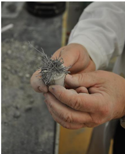
Fig. 3: Separation of fibres in under-crushed fibre-concrete by a permanent magnet
