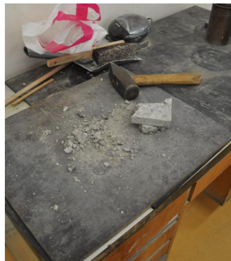
Fig. 2: Crushing of fibre-concrete specimen for precise determination of fibre concentration
