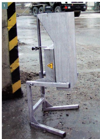
Fig. 1: Dozometer device for determination of fibre concentration in fresh concrete
