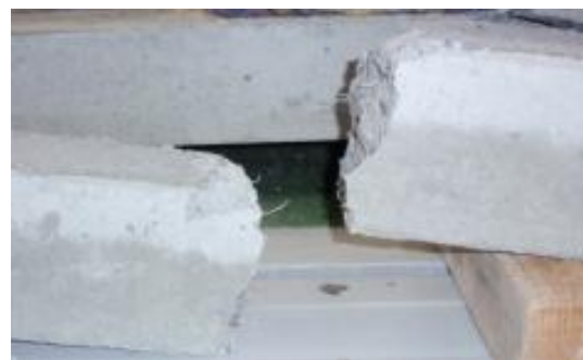
Rebars tension failure
