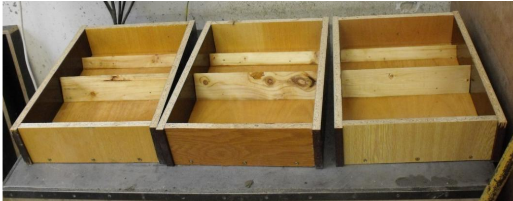
Fig. 3 Photo of forms with notches
