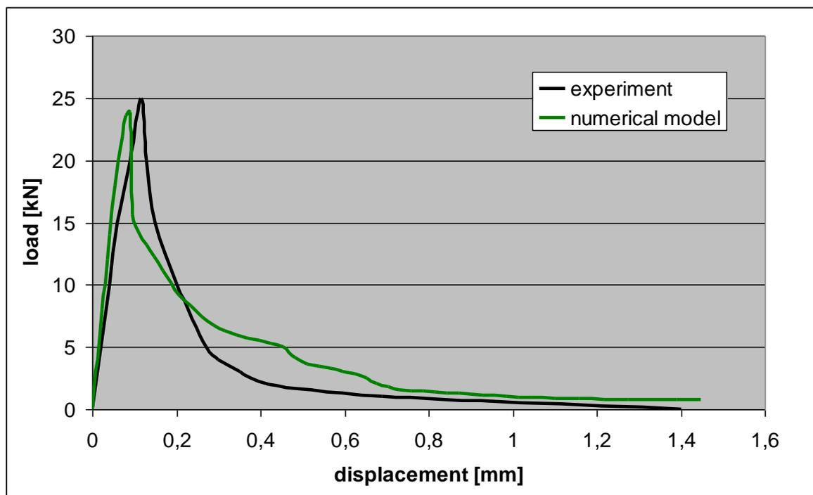
Fig. 3: Comparison of load-displacement diagrams for plain concrete beams
