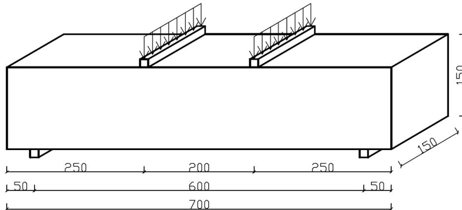
Fig. 1: Scheme of the four-point bending beam tested in [3]
