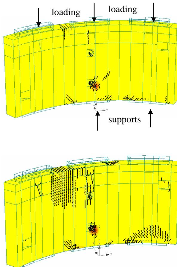
*Fig. 10:* Comparison of numerically obtained crack patterns at peak load for conventionally reinforced concrete tunnel tubing (top) and fibre reinforced concrete tunnel tubing (bottom)
