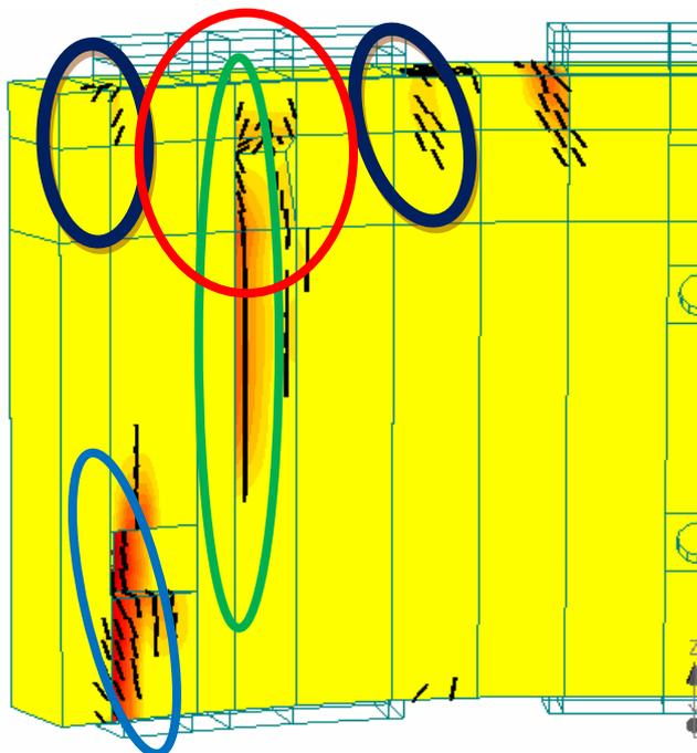
Fig. 8: Crack pattern in RC tubing in numerical simulation
