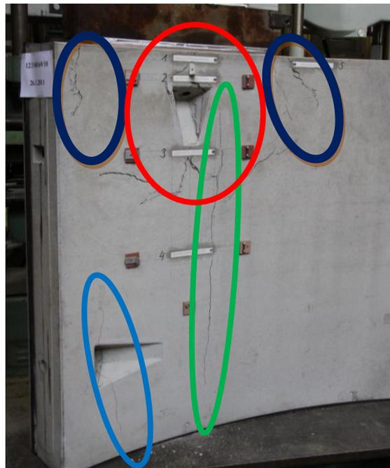
Fig. 7: Crack pattern in RC tubing in experiments
