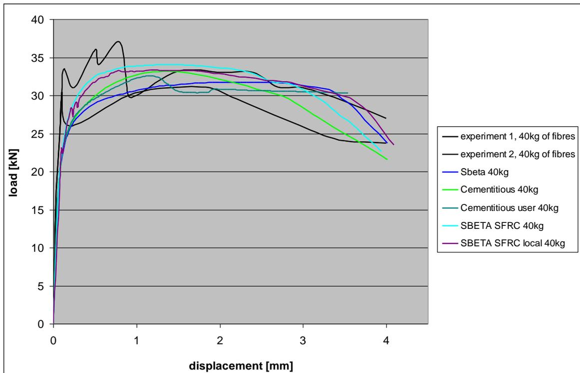
Fig. 5: Comparison of load-displacement diagrams for FRC with fibre contents of 40 kg/m<sup>3</sup>
