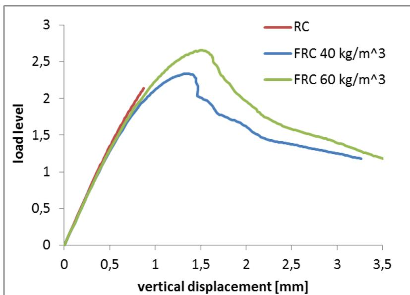
Fig. 9: Load-displacement diagram from numerical simulation of tubing – comparison of reinforced concrete and fibre reinforced concrete
