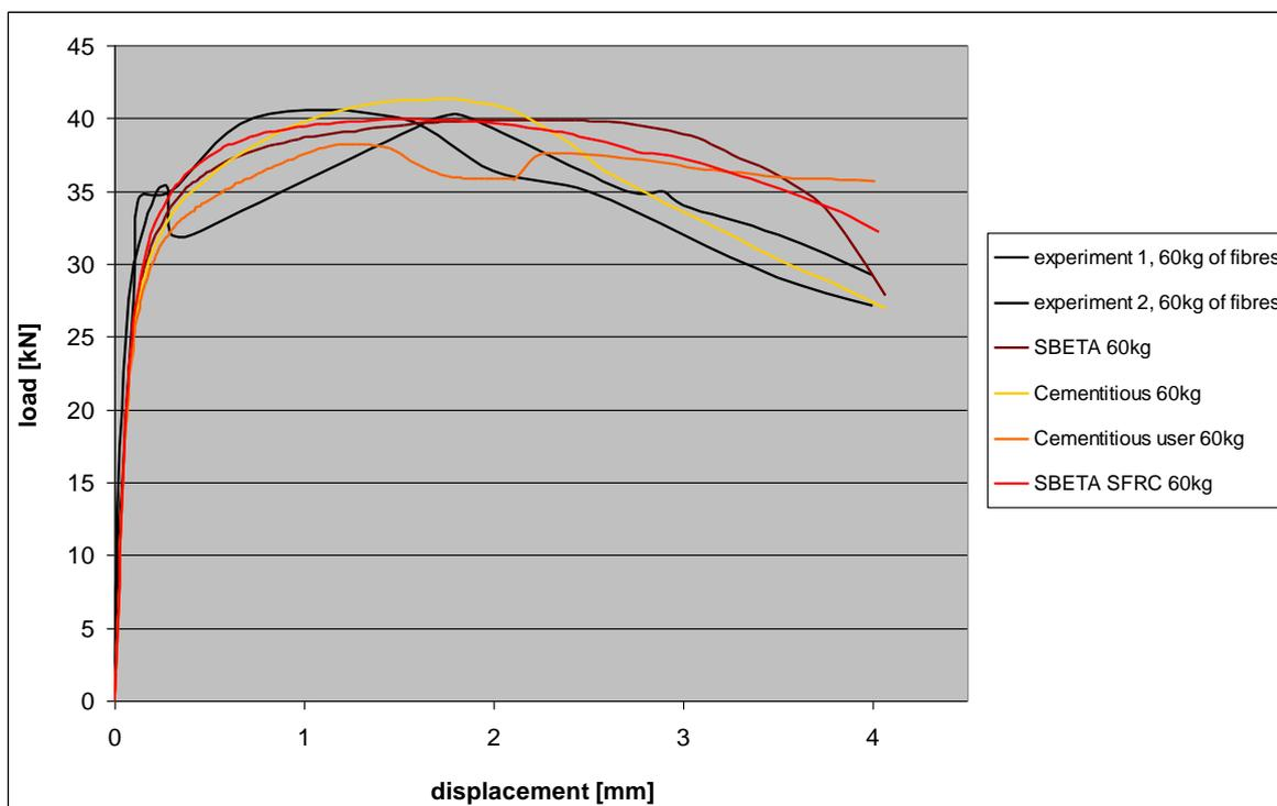
Fig. 6: Comparison of load-displacement diagrams for FRC with fibre contents of 60 kg/m<sup>3</sup>
