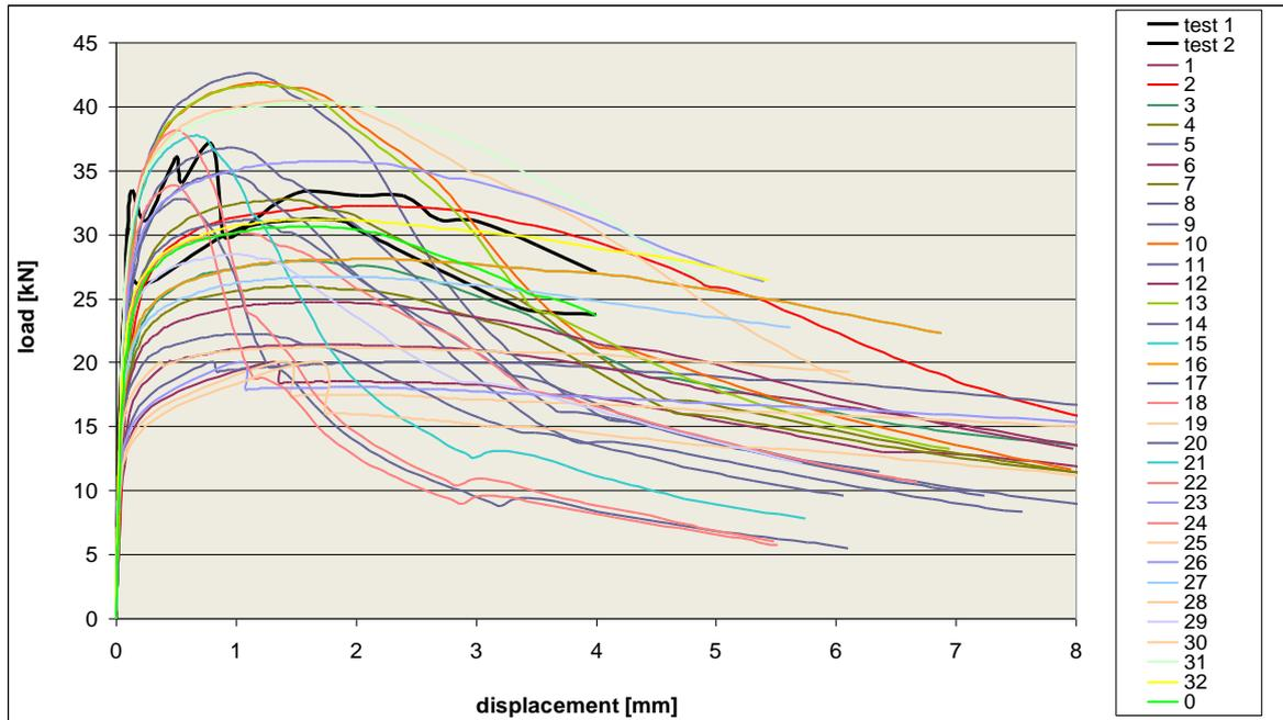
Fig. 4: Load-displacement diagrams from stochastic analysis, comparison with measured response
