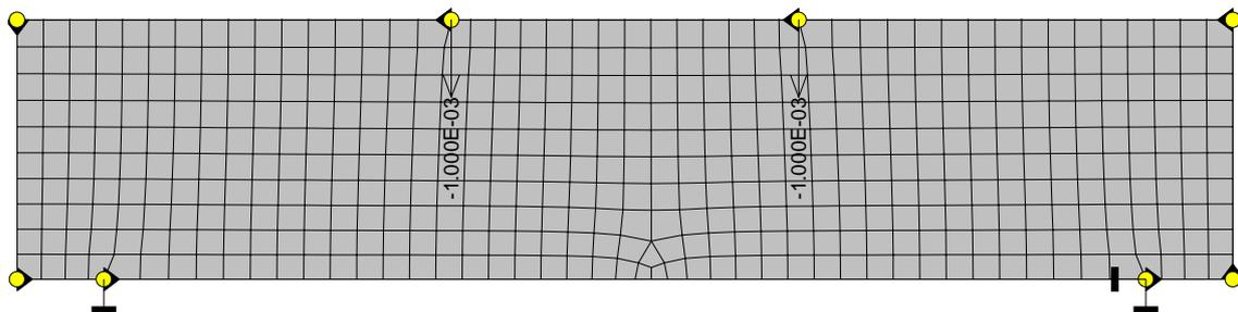
Fig. 2: Finite element model for simulation of four-point bending tests
