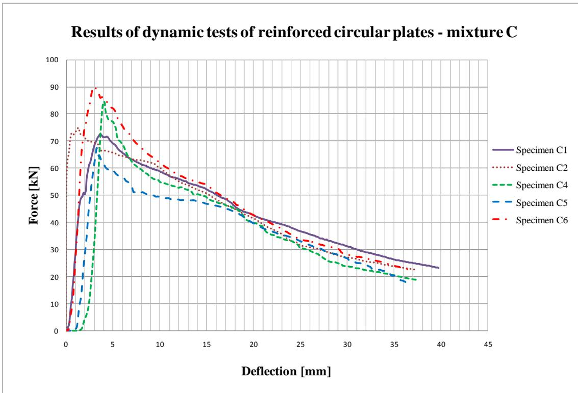
Fig. 7: Results of dynamic test of reinforced circular specimen – mixture C.
