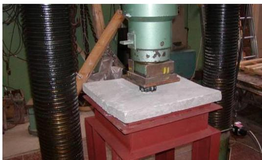
Fig. 1: Test arrangement. Square plate.
