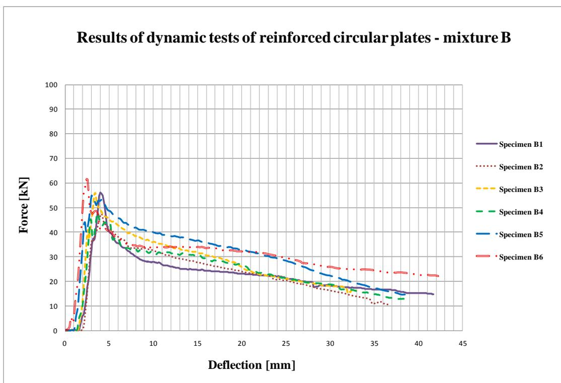
Fig. 6: Results of dynamic test of reinforced circular specimen – mixture B.
