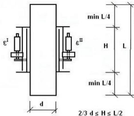
Fig. 8: Location of test equipment on test specimen.
