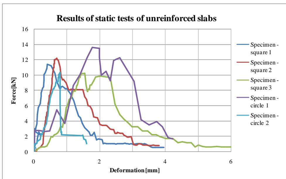
Fig. 3: Results of static test of unreinforced specimens.
