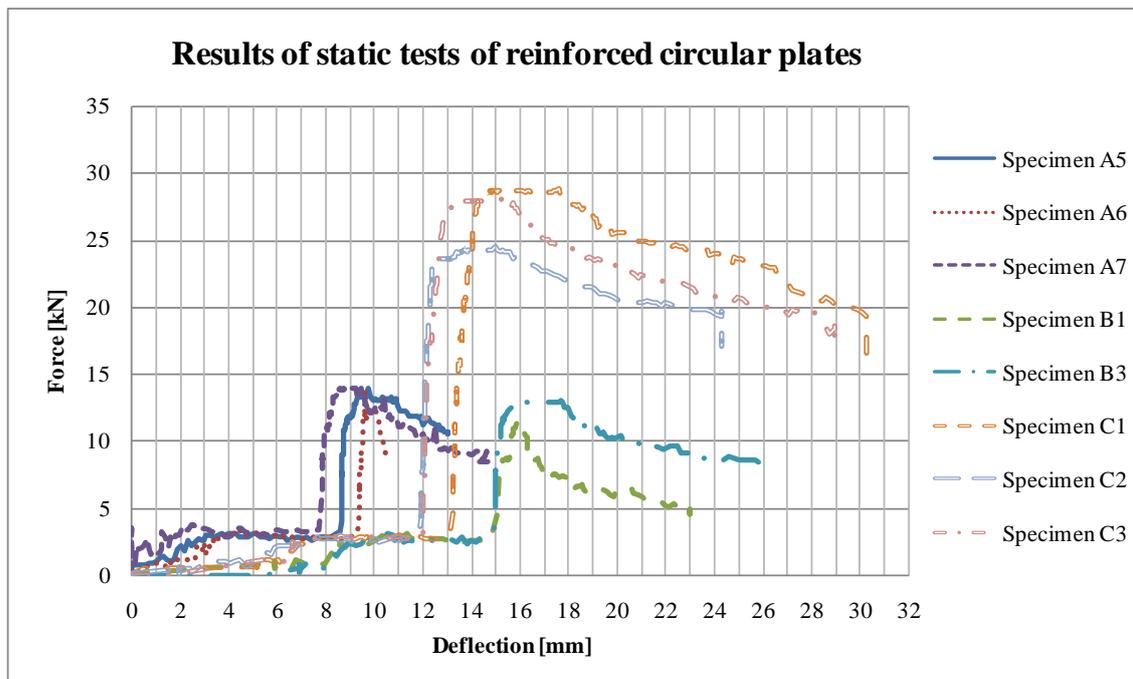
Fig. 4: Results of static test of reinforced circular specimens.
