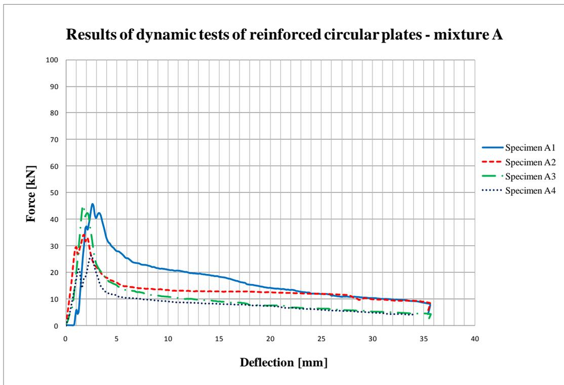
Fig. 5: Results of dynamic test of reinforced circular specimen – mixture A.
