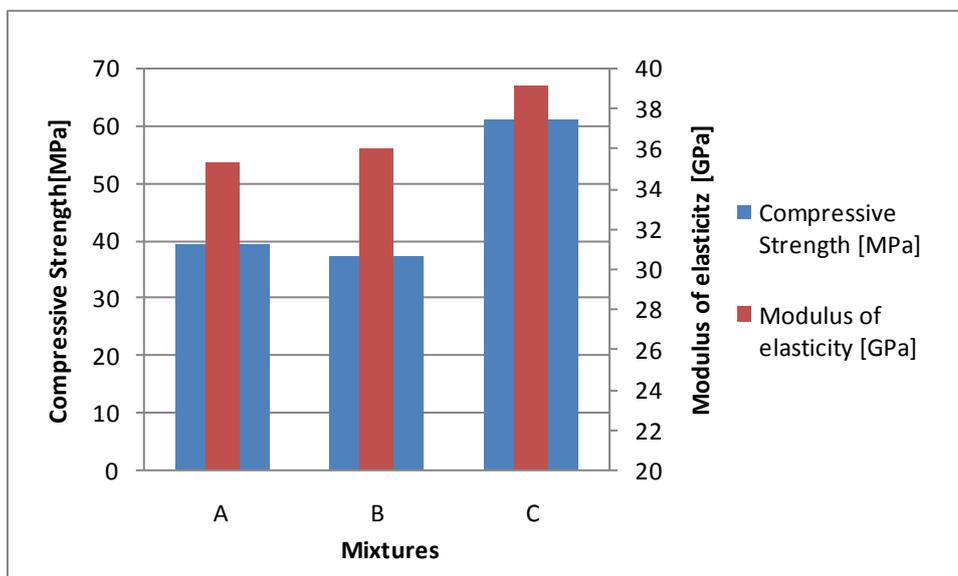
Fig. 9: Results of Modulus of elasticity and Compressive Strength.
