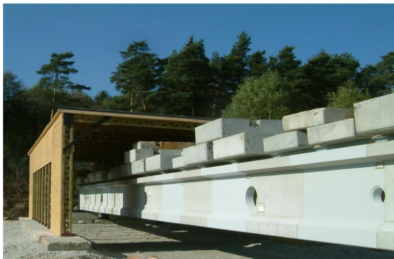
Fig. 6: Experimental beams loaded with sleeper in a continuous load test
