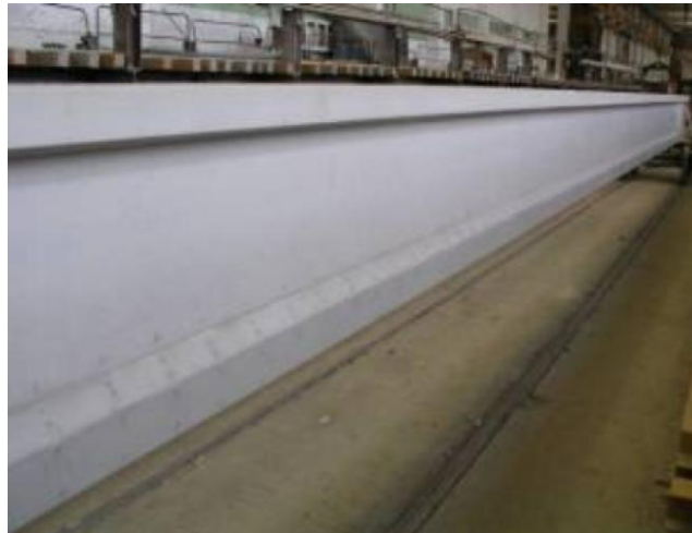
Fig. 5: The demolded girder, the blockouts at the quarter points have not yet been drilled.
