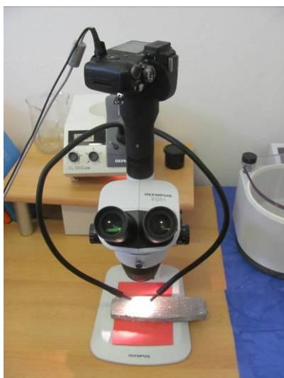
Fig. 5: The fibre distribution analysis by microscope method
