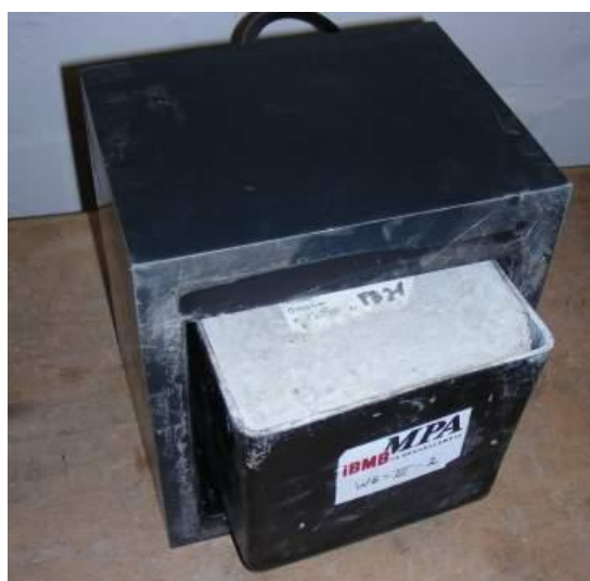
Fig. 4: Box for fresh concrete
