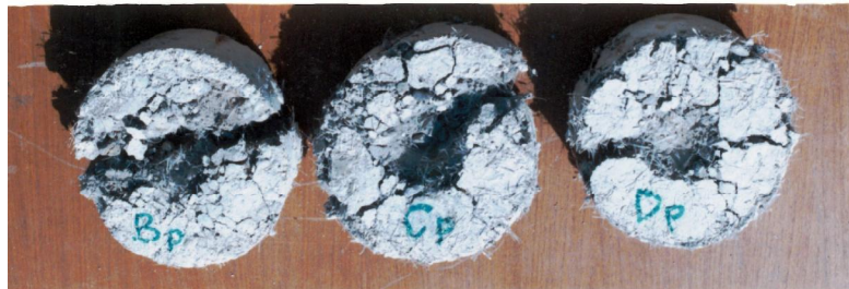
Fig. 3-B: Failure of RCC Specimens Reinforced with Polypropylene Fiber
