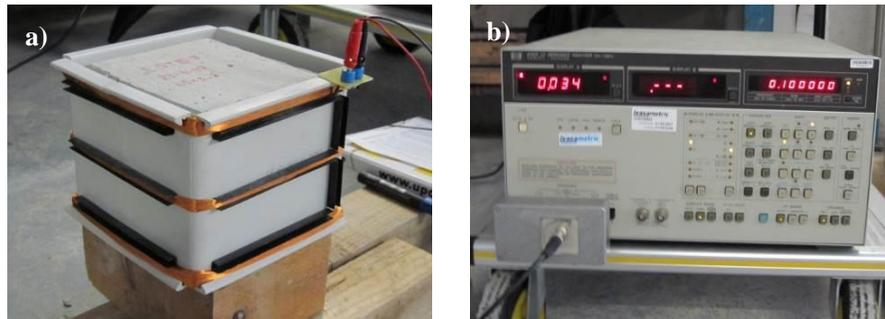
Fig. 4: Equipment of the inductive method: a) coil and b) impedance analyser.
