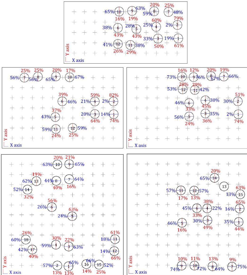
Fig. 5: Fibre orientation in specimens of: a) S\_B, b) M\_A, c) M\_B, d) L\_A and e) L\_B.
