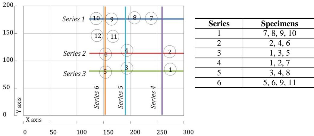
Fig. 6: Distribution of specimens in slab M\_B.
