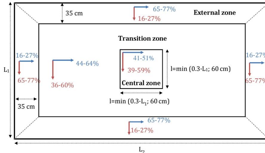
Fig. 8: Division of slabs in zones depending on fibre orientation.
