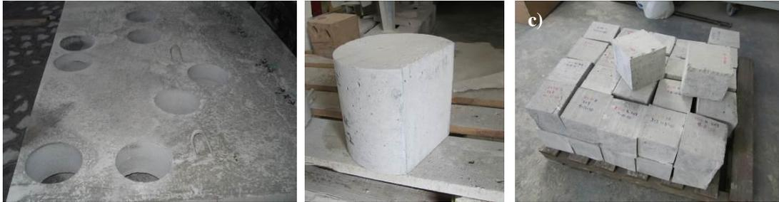
Fig. 3: a) Detail of the slab after drilling, b) cut of cylindrical cores and c) cubic specimens.
