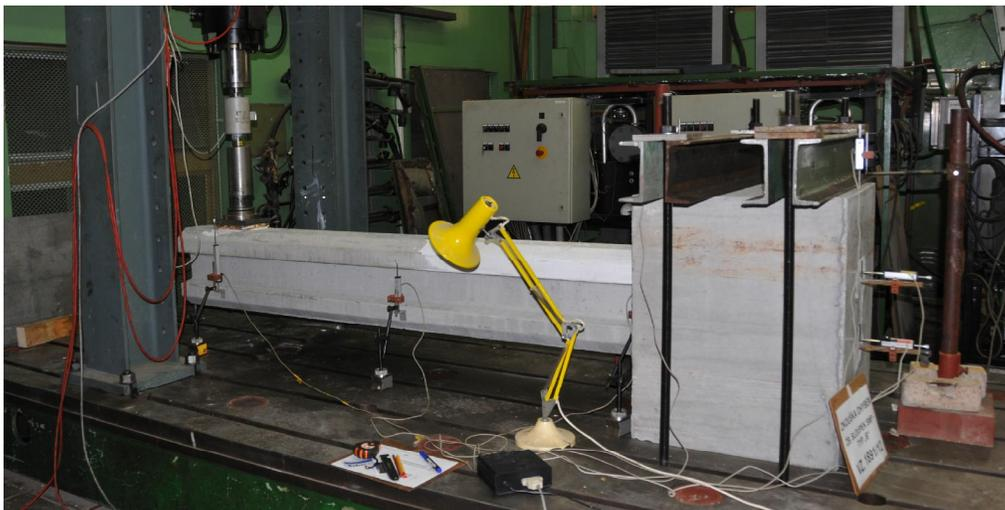
Fig. 3: Full-scale test; pier is fixed in anchoring block with height  $h_p = 600$ mm
