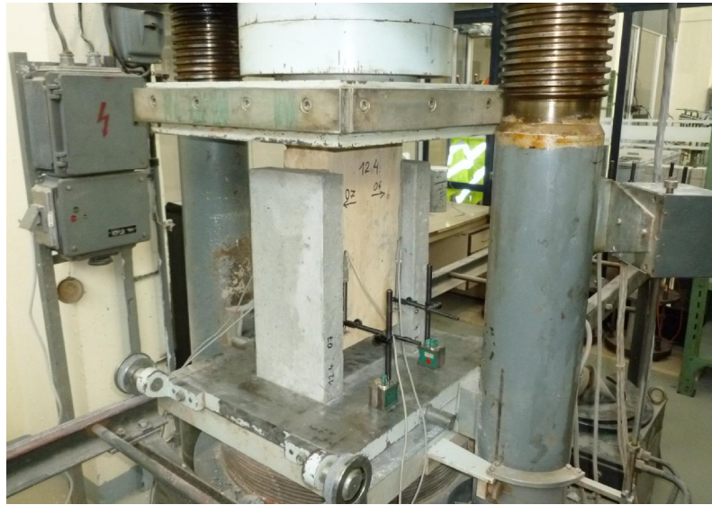
Fig. 2: Testing machine with push-out specimen
