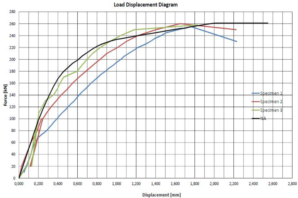
Fig. 4: Numerical model of timber-concrete composite specimen and experimental load-slip curves for A test series
