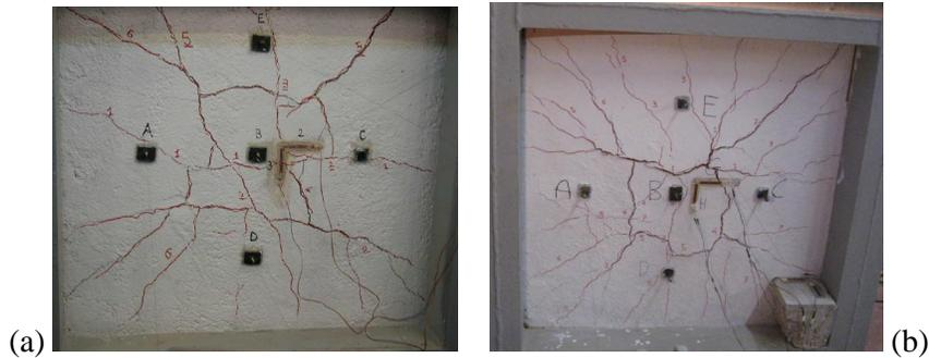
Fig. 3: Cracking failure of (a) concrete plate P1 and (b) P2
