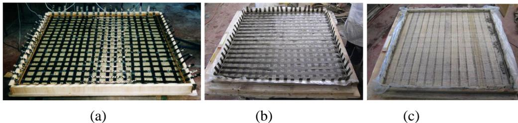
Fig. 1: Experimental plates during casting of concrete with fibre mesh: (a) carbon fibre - P1; (b) basalt fibre - P2; (c) steel fibre - P3
