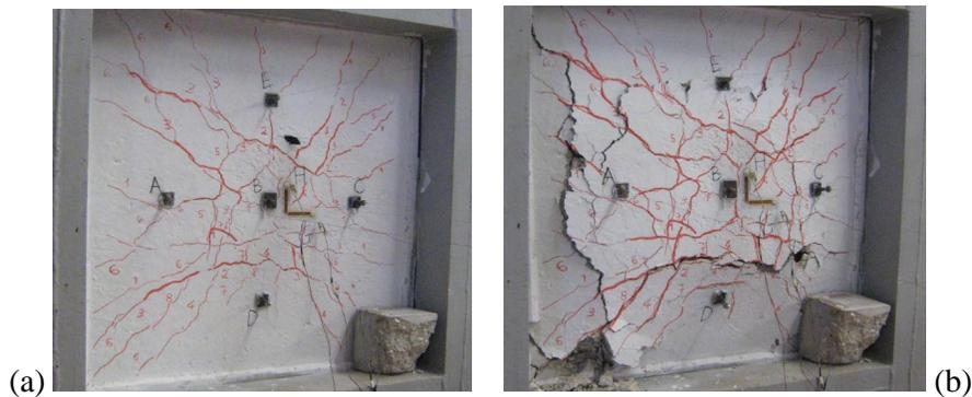
Fig. 4: (a) Cracking phase of P3 at vertical load  $P=26\text{kN}$ ; (b) punching failure.
