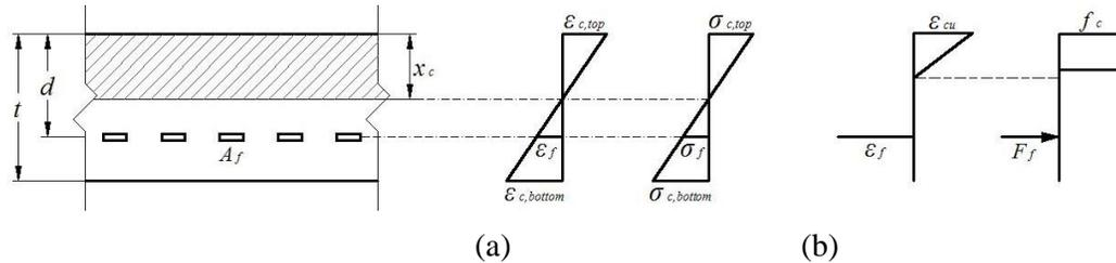
Fig. 5: Theoretical stress-strain distribution on a section of plate: (a) elastic and (b) inelastic strain-stress distribution.
