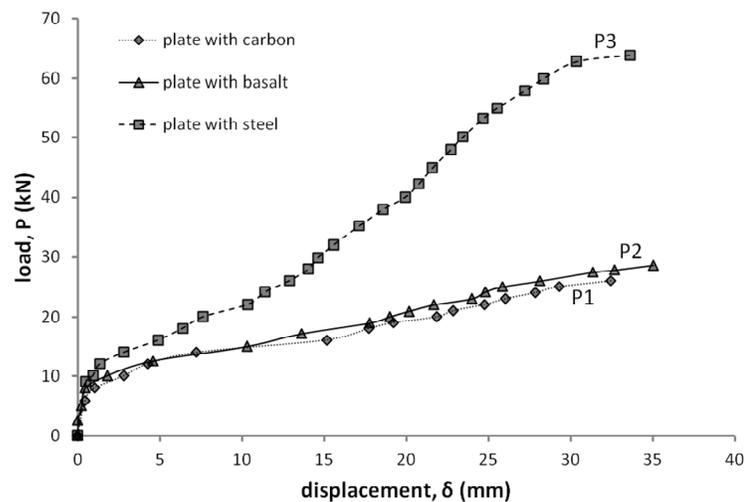
Fig. 7: Comparison of experimental load vs. displacement diagrams at the mid-point of plates P1, P2 and P3.
