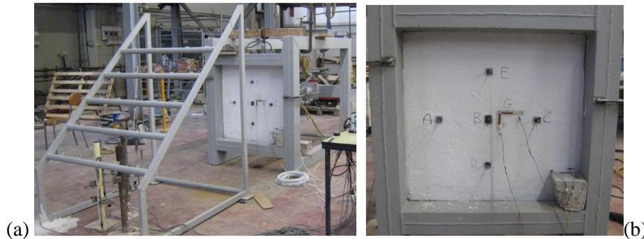
Fig. 2: (a) Set up of the concrete plates' loading tests; (b) plate surface with deflection measure points (A,...,E) and strains (G,H)
