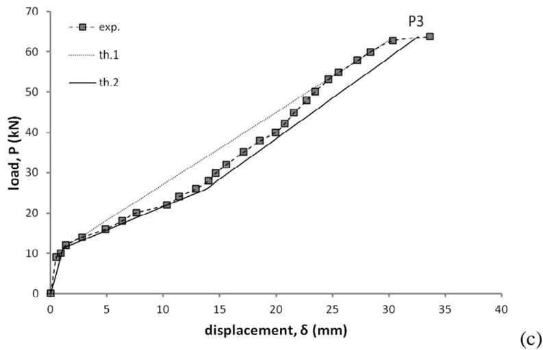
Fig. 6: Comparison between experimental and theoretical load,  $P$ , vs. displacement,  $\delta$ , for (a) P1; (b) P2 and (c) P3 plates.
