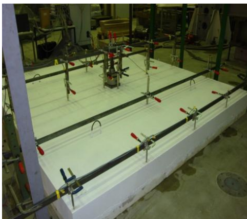
Fig. 4: Large scale testing of elastic bedded slab specimens
