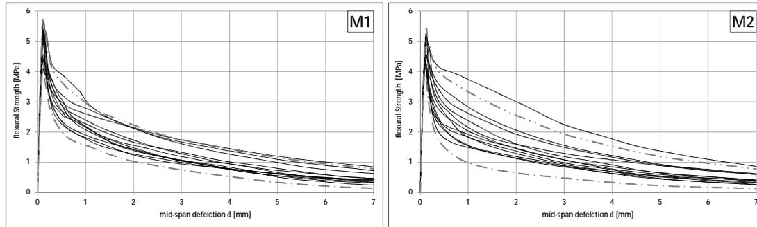
Fig. 2: Bending stress – mid-span deflection of M1 and M2 (fibre 25 mm)
