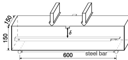
Fig. 1: Bending test specimen and setup
