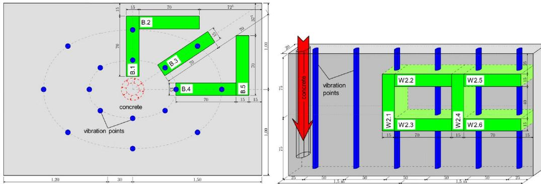
Fig. 6: Experimental setup of the basement (top view) and wall 2 and arrangements of the bending beams (equal for both walls)
