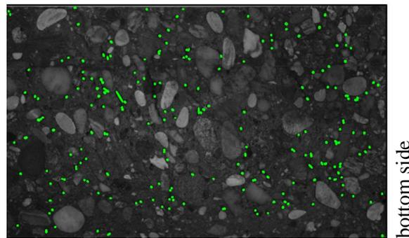
Fig. 5: Sectional area of found fibres and applied ellipses (image rotated by 90°)
