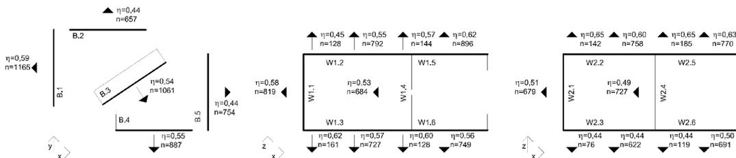
Fig. 7: Fibre orientation and number of fibres along the beams
