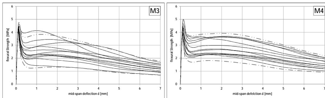
Fig. 3: Bending stress – mid-span deflection of M3 and M4 (fibre 50 mm)
