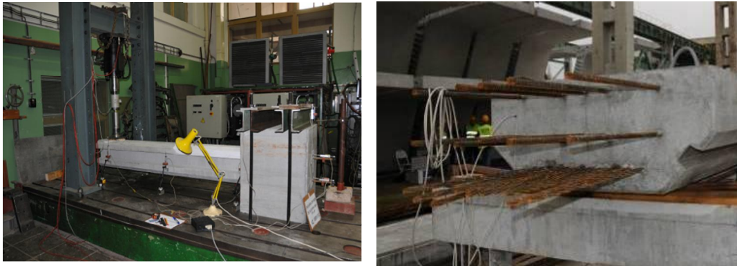
Fig. 3: Testing of prestressed elements, a) column, b) girder
