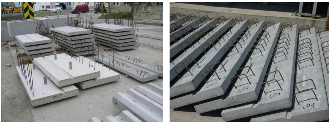
Fig. 2: (a, b) Storage of the precast plate elements
