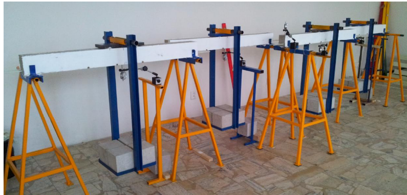
Fig. 4: Four beams (one of each series) installed for long-time loading
