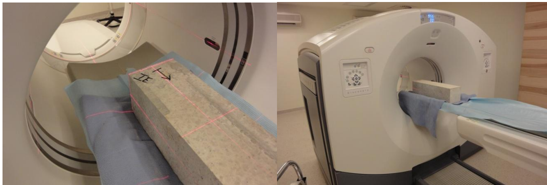
Fig. 4: The CT scanner applied for this research was equipped with 64 rows of detectors, and the thickness of a series of reconstructed native CT scan was 0.625 mm
