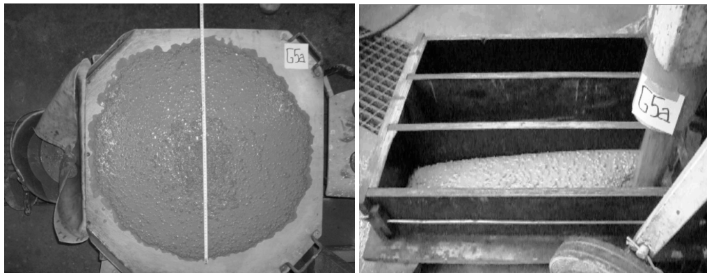
Fig. 2: Slump-flow test and forming SFRHPSCC beam C4 600x150x150 mm
