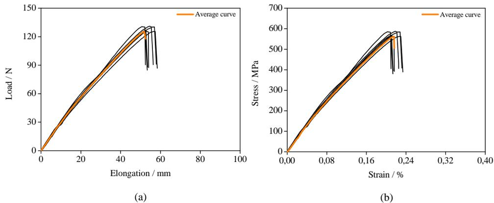
Fig. 3: Load-elongation (a) and stress-strain (b) curves.
