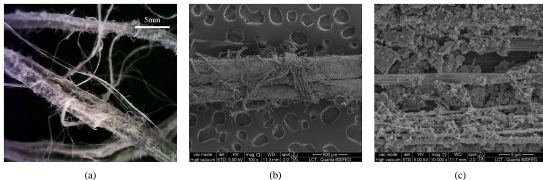
Fig. 5: Macrofiber washed out from a fresh concrete mix.
