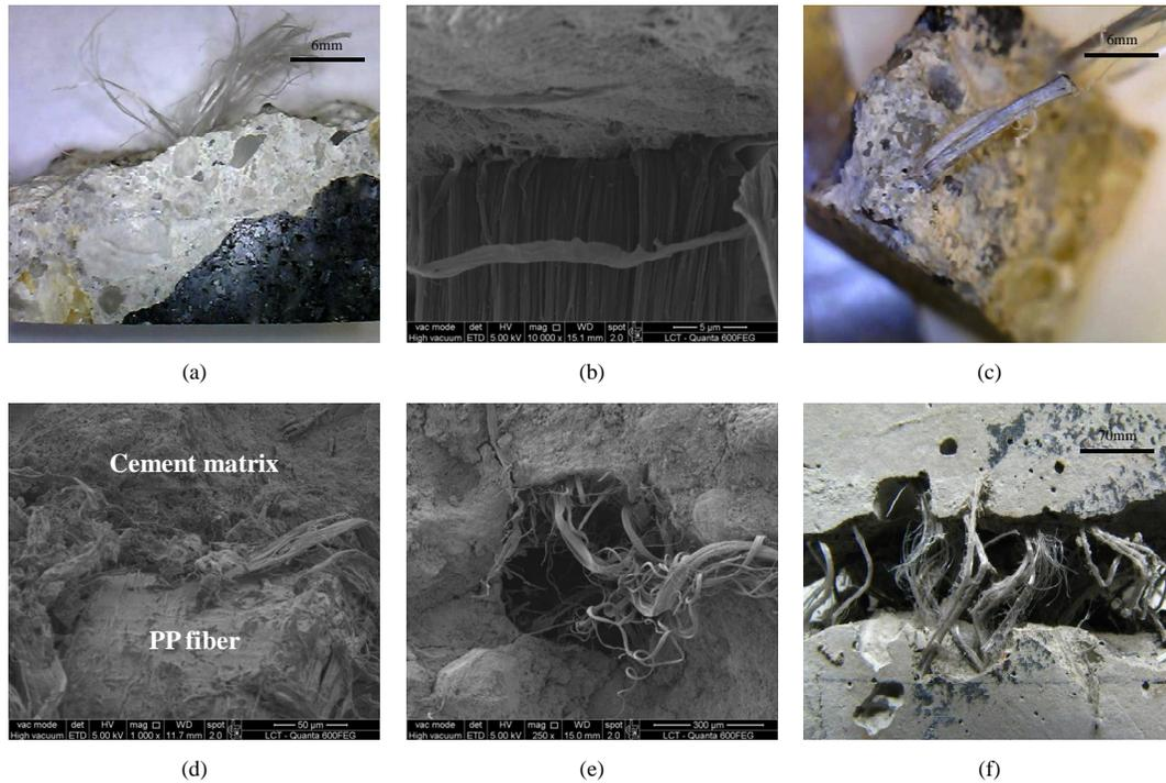
Fig. 6: Fibrillated fiber (a) and its interface with the matrix (b); Pulled-out fiber (c) and its interface with the matrix (d); void in the matrix generated by fiber pull-out (e); rupture section of a beam showing fibrillated fibers (f).
