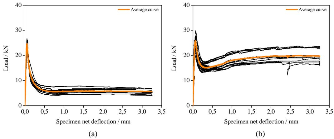
Fig. 7: Load-deflection curves obtained with concrete reinforced with fiber contents of 0.22% (a) and 1.0% (b).
