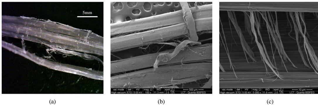
Fig. 4: Pictures of the fiber as received.
