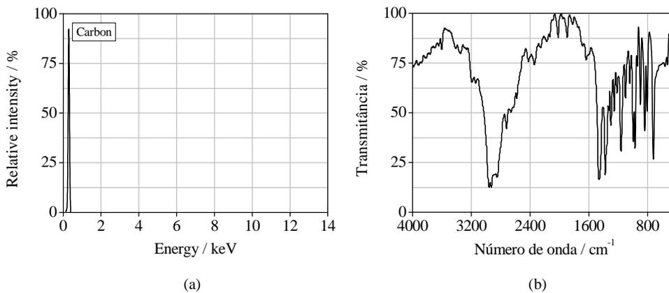
Fig. 1: EDS (a) and infrared (b) spectra of the polymeric fiber.
