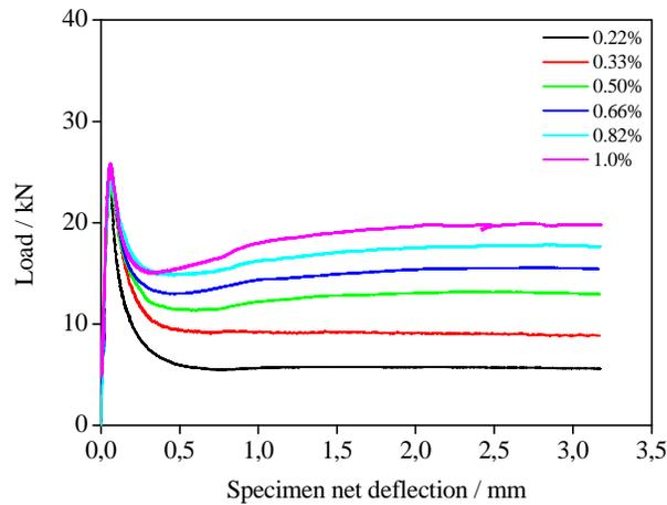
Fig. 8: Average load-deflection curves obtained with concrete reinforced with all the fiber contents used.
