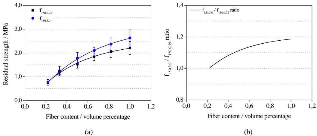
Fig. 9: Residual strengths at the deflections of 0.75 and 3.0mm (a) and ratio between them (b).
