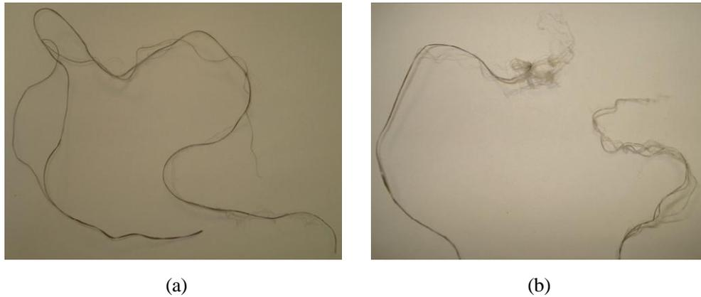
Fig. 2: Filaments after the tensile test: fibrillated (a) and ruptured (b) filaments.
