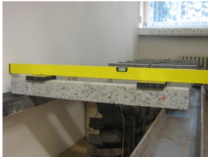
Fig. 6: Measuring of the initial deformation before the long-term loading of the specimen
