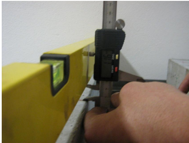
Fig. 7: Measuring of the increase of deformation
