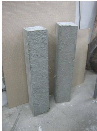
Fig. 1: Picture of the manufactured specimens 150x150x700 mm
