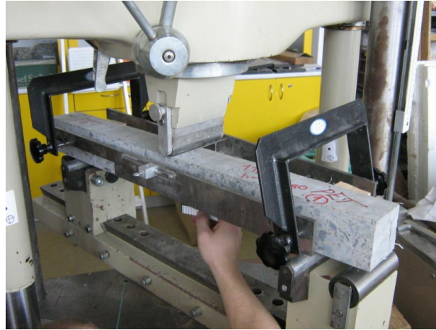
Fig. 3: Creating of a flexural macro-crack in a three-point bending test
