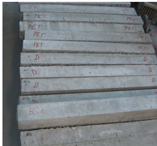
Fig. 2: Picture of the specimens for experiments 75x75x700
