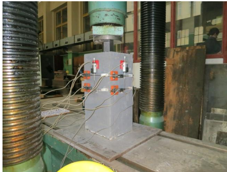
Fig. 6: Test arrangement of the anchorage zone
