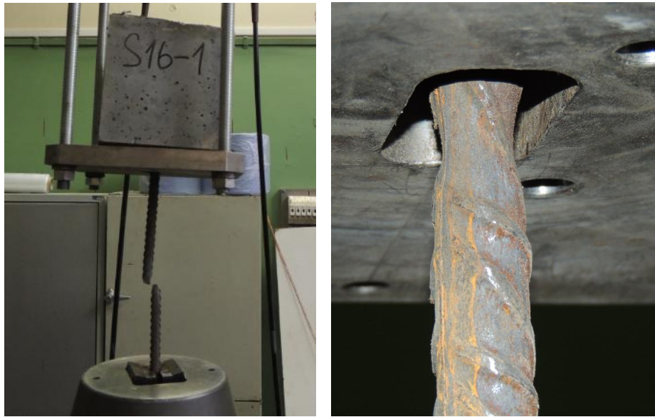
Fig. 2: Types of steel failure (specimen made from UHPC)
