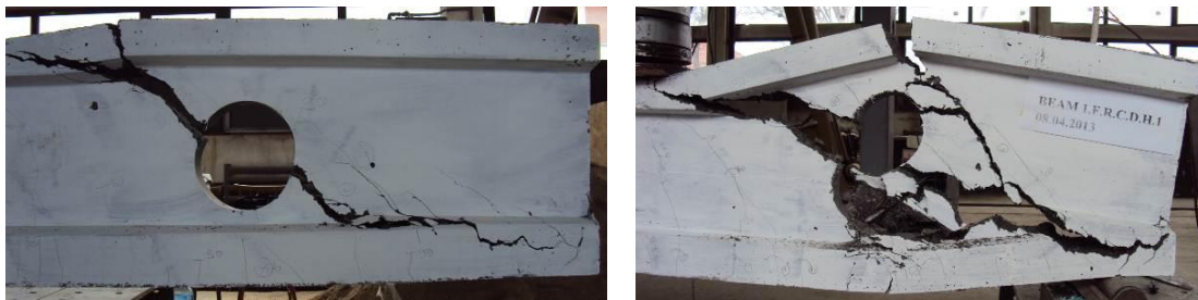
Fig. 4: Failure of FO_23.1 (left) and FOD_23.1 (right)
