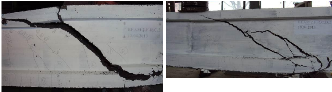
Fig. 3: Failure of F_23.1 (left) and FD_23.1 (right)
