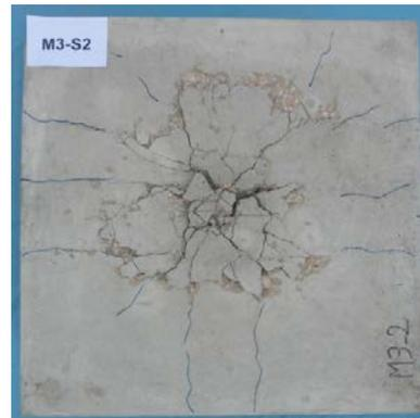
(c) Tested slab (with fiber)
