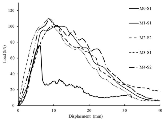
Fig. 4: Load-displacement variation for static testing of RC and HFRC slabs
