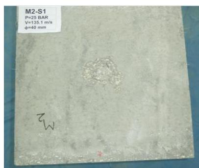
(e) Slab with fibers (Front face)
