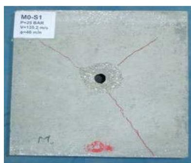
(c) Slab without fibers (Front face)
