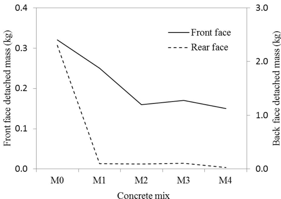
Fig. 7: The ejected concrete mass impacted by the projectile at impact velocity of 135 m/s.
