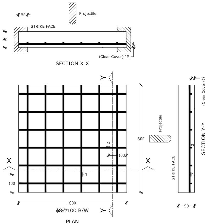
Fig. 1: Reinforcement and instrumentation details of the concrete slabs
