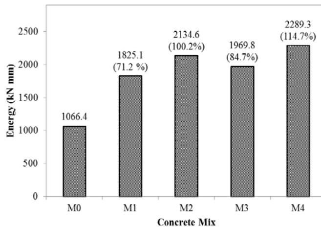
Fig. 6: Energy absorption in punching of control and HFRC slabs
