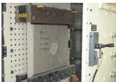
(a) Slab without fibers (Front face)
