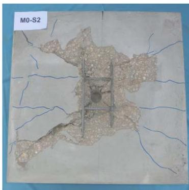
(b) Tested slab (no fiber)
