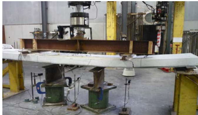
Fig. 8: Typical slab failure
