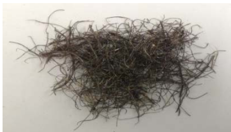
Fig. 1: Recycled steel fibres extracted from wasted tires
